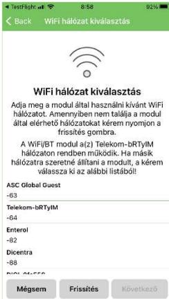
Within 15 minutes, the **Cloud Manager** application must be started and then the module must be paired with a Bluetooth connection. After setting up Bluetooth, you can connect your module to the local WIFI network. At the end of the WIFI setup, it will automatically restart and connect to the configured WIFI network. When connected successfully, you will see a green LED. It will try up to 20 times if the connection fails.
