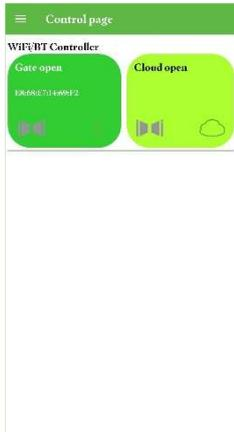
The parameters of the module can be set via the Cloud Manager mobile application with Bluetooth connection or in case of WIFI network access at [www.ascloudmanager.com](http://www.ascloudmanager.com). After setting up properly in the Cloud Manager application, you can also control your devices with a Bluetooth or Cloud (connected to a WIFI or Internet network) icon. For individual icons, grouping them in different colors can make output control even easier.
