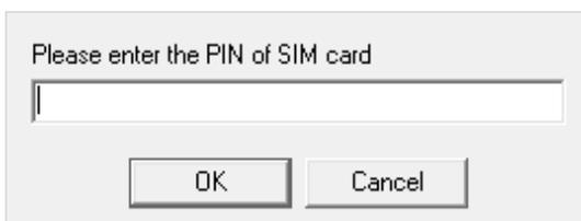
Before inserting SIM card in the module the PIN code request should be switched off
