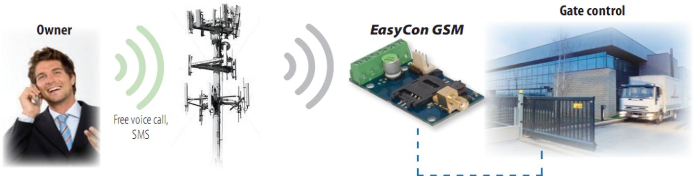
Figure 1: Device operation
