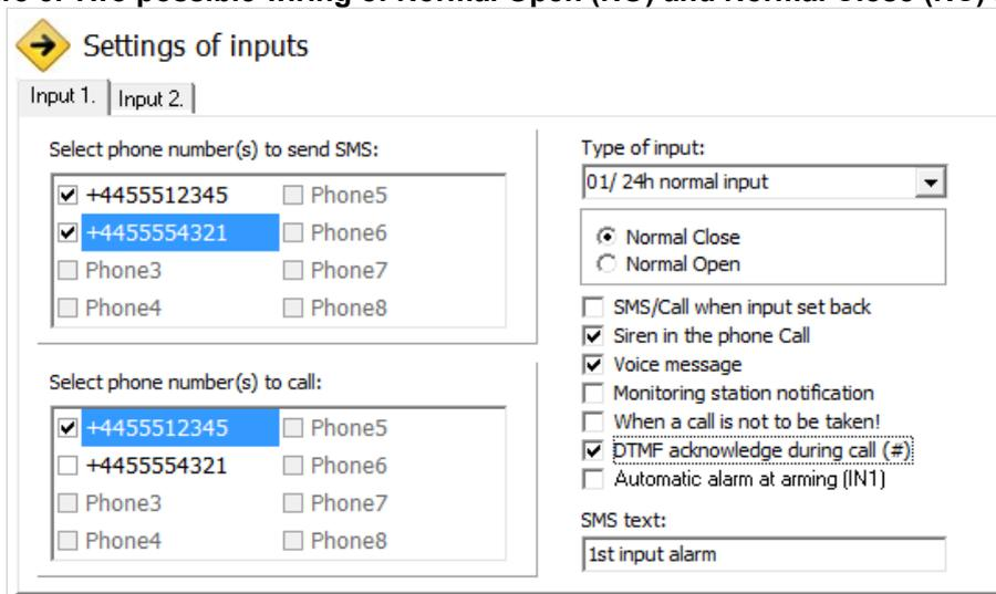
You can set on this tab if there is an alarm event caused by short or open circuit on an input to which phone number you would like to send SMS or voice message notification. It is possible to send both notifications to the same phone number.
