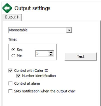
On the **Output** window the output settings can be changed. The output type can be *monostable* namely one stasured, (switches off for the given period than reverts back to the original status), or *bistable* namely two stasured (it only will revert back to original state after a new controlling).
