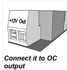
The OC relay has to be connected directly through its “+12V” and “Out” series terminal with EasyCon GSM power source and with the (O) output.
