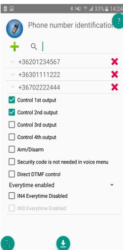
By choosing the „Caller ID” option, we can save phone numbers to the memory of the module. First the module reads out the phone numbers from the memory. Afterwards, we can give the numbers along with assigning the different functions like arming/disarming or controlling output 2. We can store up to 1000 phone numbers.
