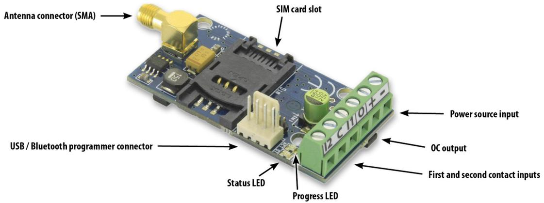
Figure 2: The buildup of the module
