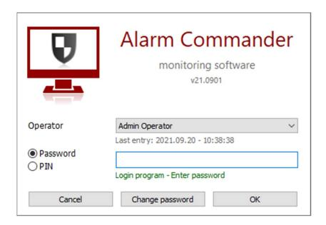
**After a new installation,** a default operator with administrator rights can be chosen for login. The default **password is 1**, the default **PIN code** is **1234**.
