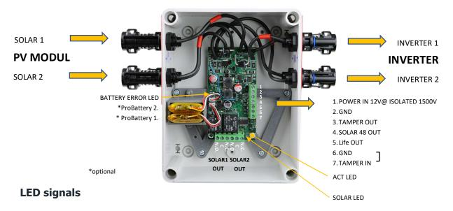
The red LED (ACU LED) next to the battery lights up, indicating that it is probably necessary to replace the internal battery. The system cannot report a bad battery if an external power supply is used. The LED's at the terminals show the signals of the corresponding outputs, the LED lights up when active.
